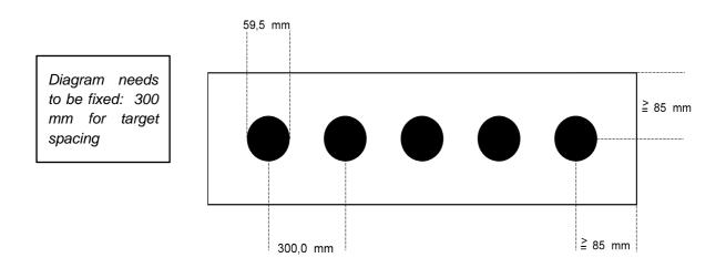
The Diameter of the black is 59.5 mm with a tolerance of +0.2 mm / - 0.0 mm
